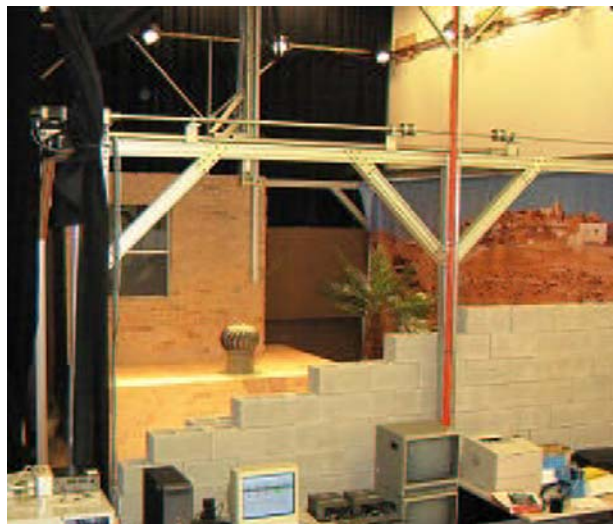
Fig. 4 Systems Integrated Sensor Test Rig (SISTR). SISTR provides a stage for testing and evaluation of hardware in simulated urban environments and disaster scenarios. Effects such as varied lighting, rain, fog and smoke can be introduced in a controlled and repeatable fashion
