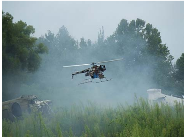
Fig. 1 The SR100 robotic rotorcraft hovers over an unsafe landing site. A laser range finder mounted to the bottom of the craft is tested for its performance in smoke
