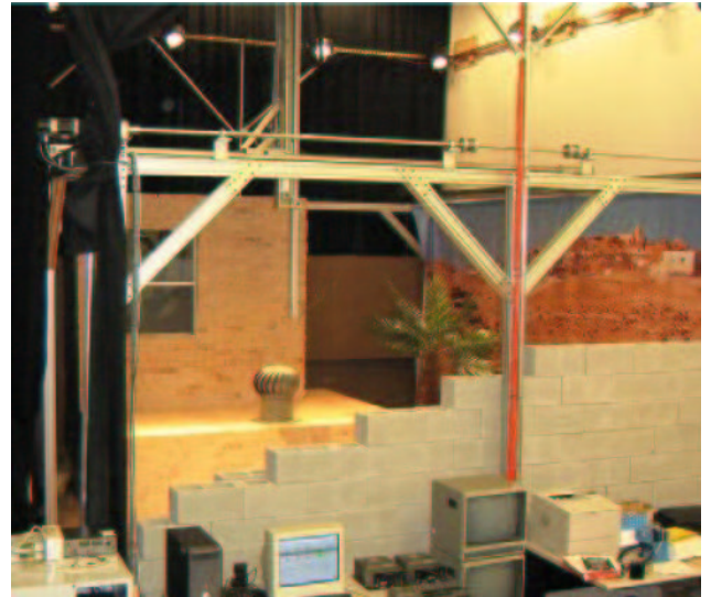
Figure 4. SYSTEMS INTEGRATED SENSOR TEST RIG (SISTR). SISTR PROVIDES A STAGE FOR TESTING AND EVALUATING SENSOR AND CONTROL ALGORITHMS IN A SCALED ENVIRONMENT. THE 6 DOF GANTRY THAT COMPRISES SISTR CAN BE PROGRAMMED THROUGH MODEL ADAPTIVE CONTROL TO MIMIC THE FLIGHT OF UAVS.
