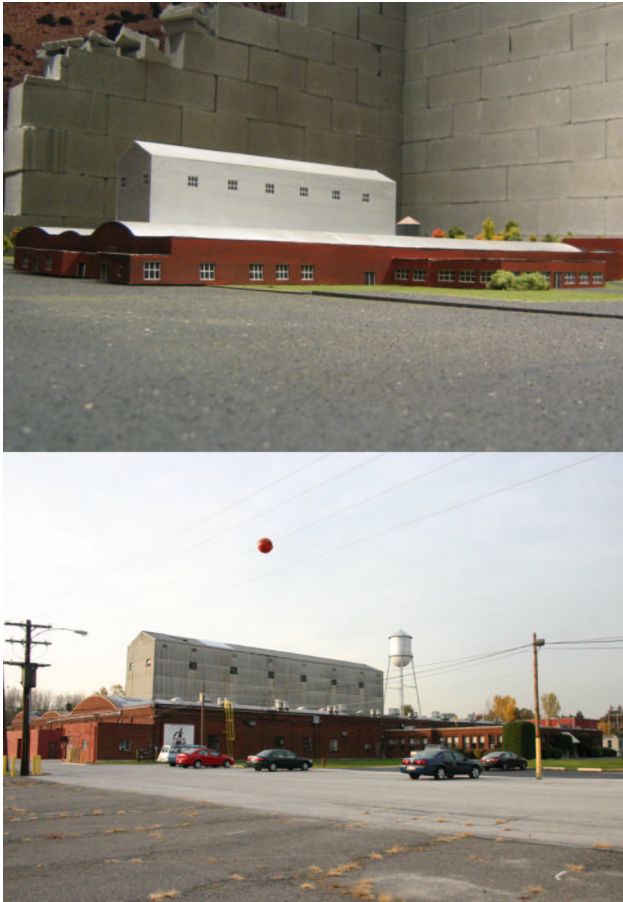
Figure 3. THE V&V ENVIRONMENT COMPARED TO THE 1/87TH SCALE T&E ENVIRONMENT. THE T&E FACILITY WAS CREATED TO CLOSELY APPROXIMATE THE HELICOPTER DEVELOPMENT RANGE IN ORDER TO DRAW A CONTINUOUS PATH BETWEEN LABORATORY TESTING AND REAL-WORLD FLIGHTS.
