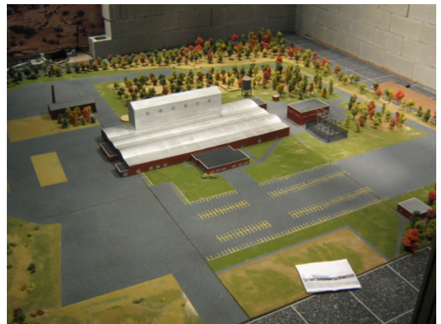
Figure 1. A SCALED MODEL ENVIRONMENT FOR TESTING UAV MISSIONS. THINGS SUCH AS TREES AND UNSTRUCTURED LIGHTING THAT ARE DIFFICULT TO CAPTURE IN COMPUTER SIMULATION ARE EASILY INCORPORATED HERE.
