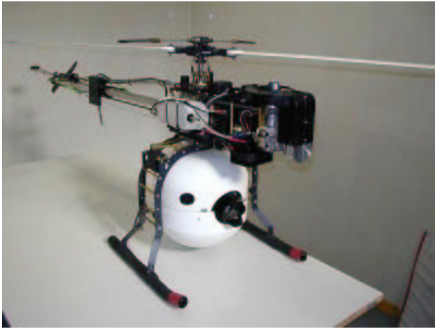
Figure 5. THE SR100 HELICOPTER FROM ROTOMOTION, INC. THE SR100 IS SOLD AS A FULLY ROBOTIC PACKAGE CAPABLE OF AUTOMATED TAKE OFF, LANDING, AND GPS WAYPOINT FOLLOWING.
