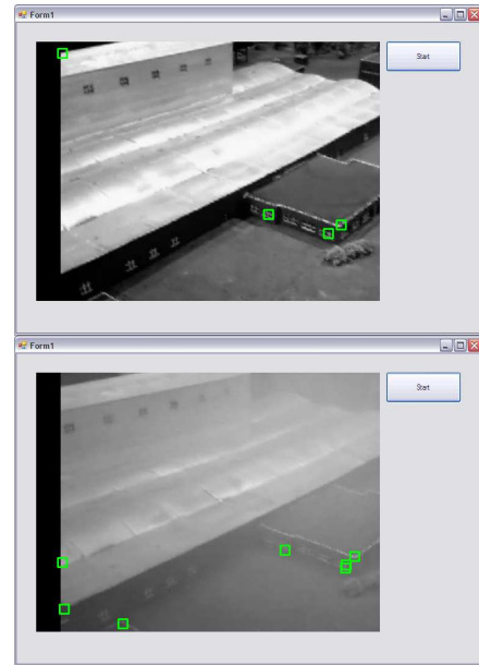
Figure 12. KLT tracking was also performed in an environment obscured with fog. The image became more washed-out, but the same features were still detected. These features were weaker than those found in the unobscured image, making them more difficult to track.
