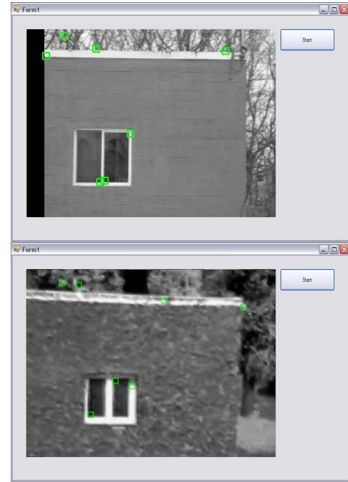
Figure 8. A Kanade-Lucas-Tomasi feature tracker was applied to video from the scaled model and the real world. Similar features were detected and tracked in both data sets. This confirms that vision sensors produce similar results at both small and full scale.
