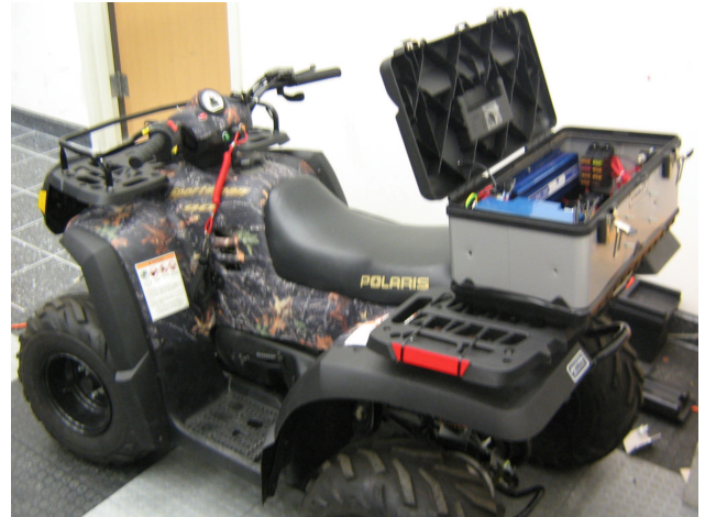
Figure 1: Drexel's Integrated ATV System (DIAS). Project DIAS is a robotic retrofit for a stock ATV. Pictured here is DIAS-2, a converted Polaris Sportsman 90cc with electronics bay on the back rack.
